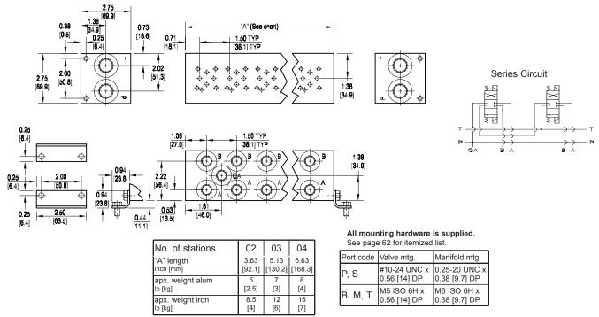
Note: Both Daman's parallel and series D02 manifolds have pressure and tank lines that run the length of the manifold. Consequently it is commonly assumed that an error was made by marking a parallel manifold incorrectly as a series. Upon closer inspection it can be seen that the valve patterns are indeed connected in series.
